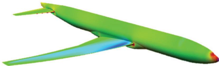
**Figure 1.** Pressure at the surface of a commercial aircraft computed using model order reduction. From K. Washabaugh, D. Amsallem, M. Zahr, and C. Farhat, *Nonlinear Model Reduction for CFD Problems Using Local Reduced-Order Bases*, 42nd AIAA Fluid Dynamics Conference and Exhibit, June 25–28, 2012, New Orleans, Louisiana.
