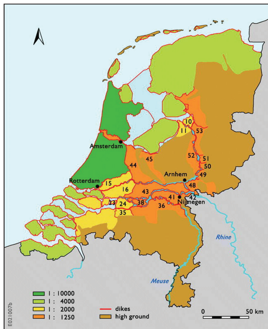
Figure 1. Dike-ring areas in the Netherlands, color-coded according to flood protection standards. From Klijn, van Buuren, and van Rooij (2004) / Rijkswaterstaat [7].
