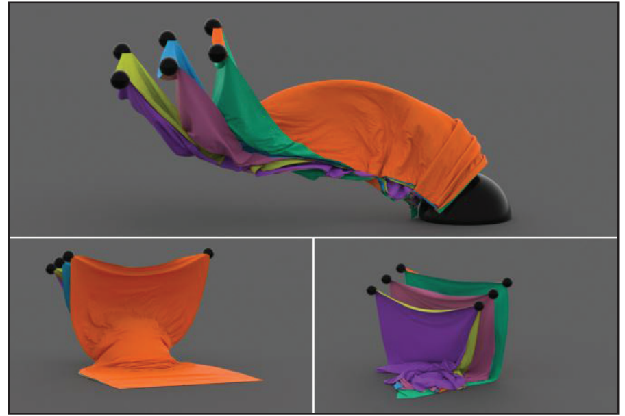
Figure 2. A sphere pushes three pieces of cloth—with approximately 1.4 million triangles—back and forth. This yields complex folds and contact. Image courtesy of [1].
