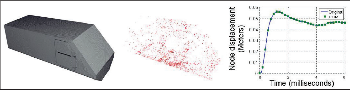
Figure 1. Simulating the underbody blast of a V-hull vehicle with a ROM. Original computational domain with 2.4 \times 10^5 elements (left), subset of the domain with 2 \times 10^3 elements used by the ROM (center), and a comparison of the results (right). The ROM generated sub-1% displacement errors with a 10^4 wall-time speedup. Courtesy C. Farhat.
