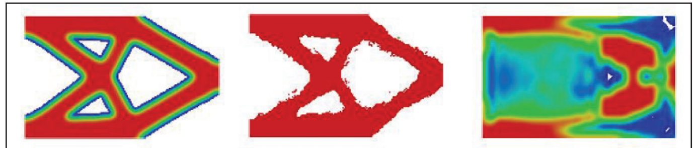
Figure 2. Topology optimization with reduced-order models. Optimal solution (left), ROM-based optimization solution after 2000 seconds (center), high-fidelity-model-based optimization after 2000 seconds (right). Courtesy M. Zahr.
