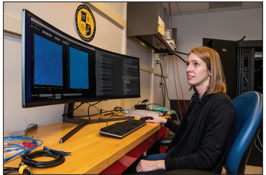
Tegan Webster, a mathematician at the U.S. Naval Research Laboratory (NRL) and head of the Radar Division's Distributed Sensing Section, analyzes the graphical user interface of the Multichannel Active Electronically Scanned Array (MAESA) radar testbed in Washington, D.C. The MAESA system transmits, receives, processes, and visualizes data for research and development in radar technology. U.S. Navy photo courtesy of Sarah Peterson.
