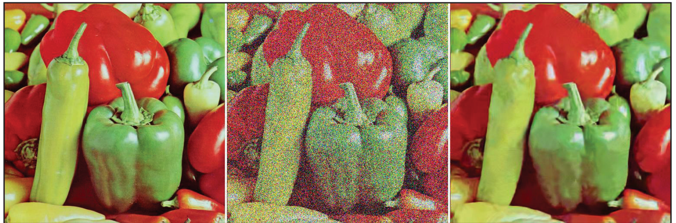
Figure 2. A denoising example. Left. An original image (public domain). Middle. Image contaminated by additive Gaussian noise of STD=100 . Right. The denoising outcome obtained by one of the leading algorithms — the BM3D [1]. Image credit: Michael Elad.
